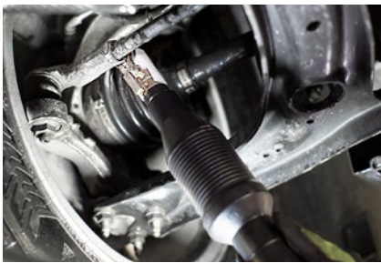
WHEEL ALIGNMENT APPLICATION LOOSEN TIE ROD NUTS SAFELY
