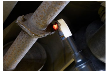
SERVICE APPLICATION REMOVE RUSTY EXHAUST BOLT
